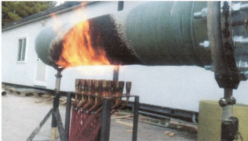
Picture No. 5: Fire endurance test. Test time 10 min.
