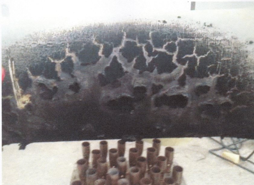
Picture no. 9: The test specimen after the fire endurance test. The exposed face of the pipe
