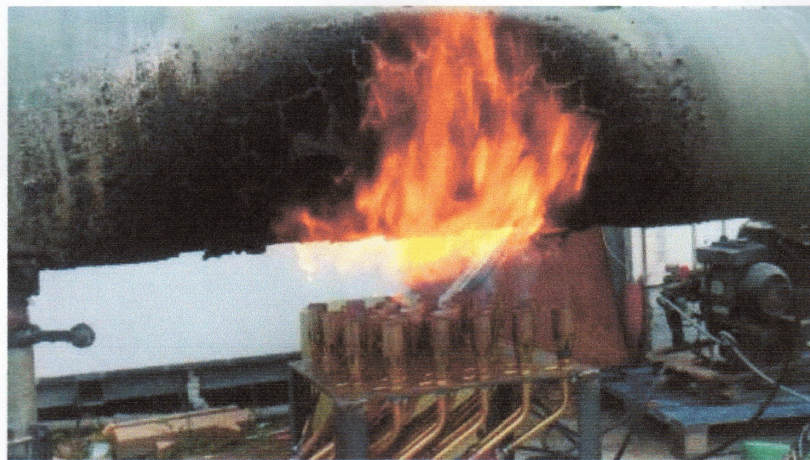
Picture no. 7: Fire endurance test. Detail (Test time 18 min.)
