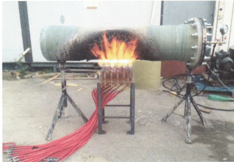
Picture no. 8: Fire endurance test. Test time 25 min.
