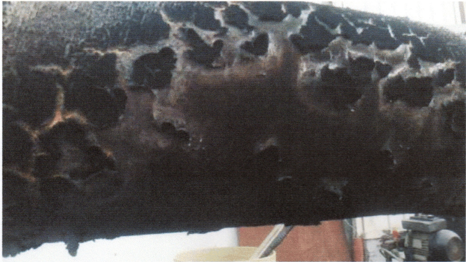
Picture no. 10: The test specimen after the fire endurance test. The exposed face of the pipe
