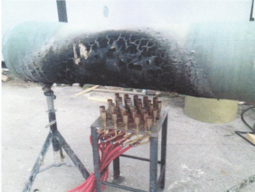
Picture no. 12: Test Specimen during pressure test (no leakage observed)
