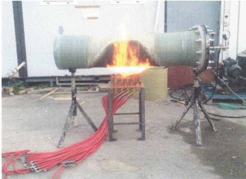
Picture No. 4: Fire endurance test. Test time 5 min.
